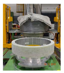
Figure 5. Shrink-fitting operation at ASG premises
