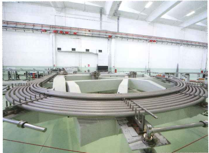
Winding the final conductor for Europe's ITER Toroidal coils, ASG Superconductors, La Spezia, Italy
